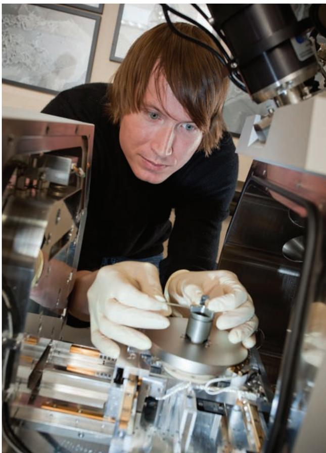
**Postdoctoral fellow Mark Curtis prepares a sample for the focused ion beam scanning electron microscope used to examine the smallest details within shale. He works in the Devon Nanolab with equipment donated by the oil company in 2010.**
